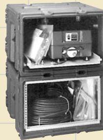
RF-382A-15TM 400-Watt Antenna Coupler Mini-Transit Case System
